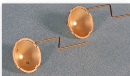
Density determination sets for solids DSS 11 and DSS 12
