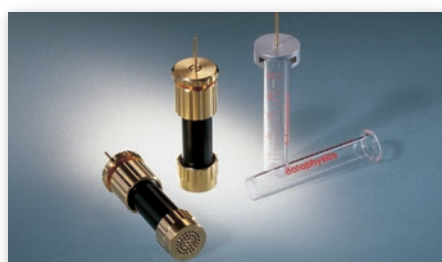
Holders for fibre bundles FH 11 and for powders PUR 11
