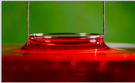
Du Noüy ring with liquid lamella
