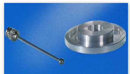
Fig. 3: Sample vessel and test piece for lamella method
